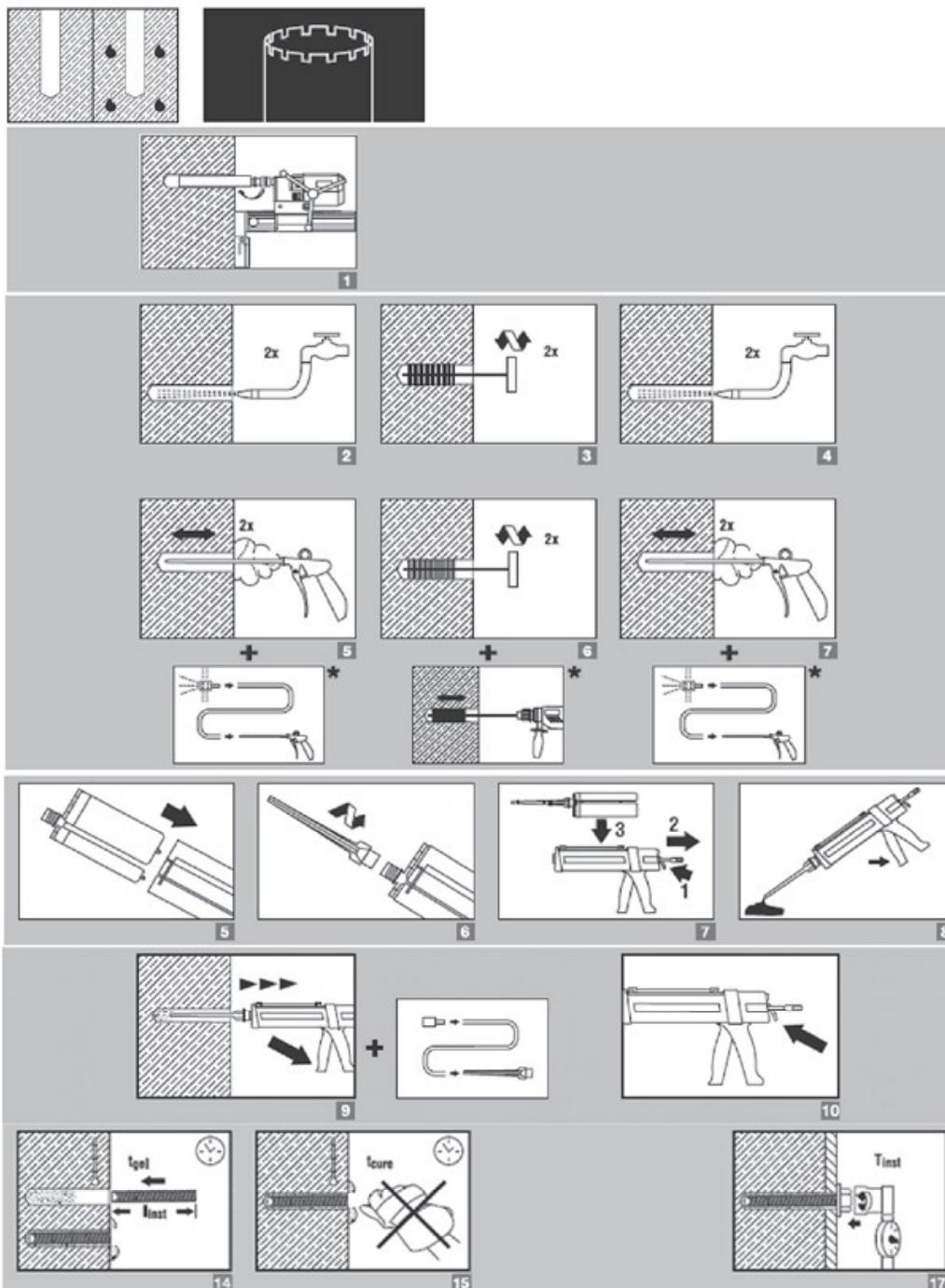
**For anchors in diamond drilled holes load values for combined pull-out and concrete cone resistance have to be reduced. Load reduction factor: 0.7**
