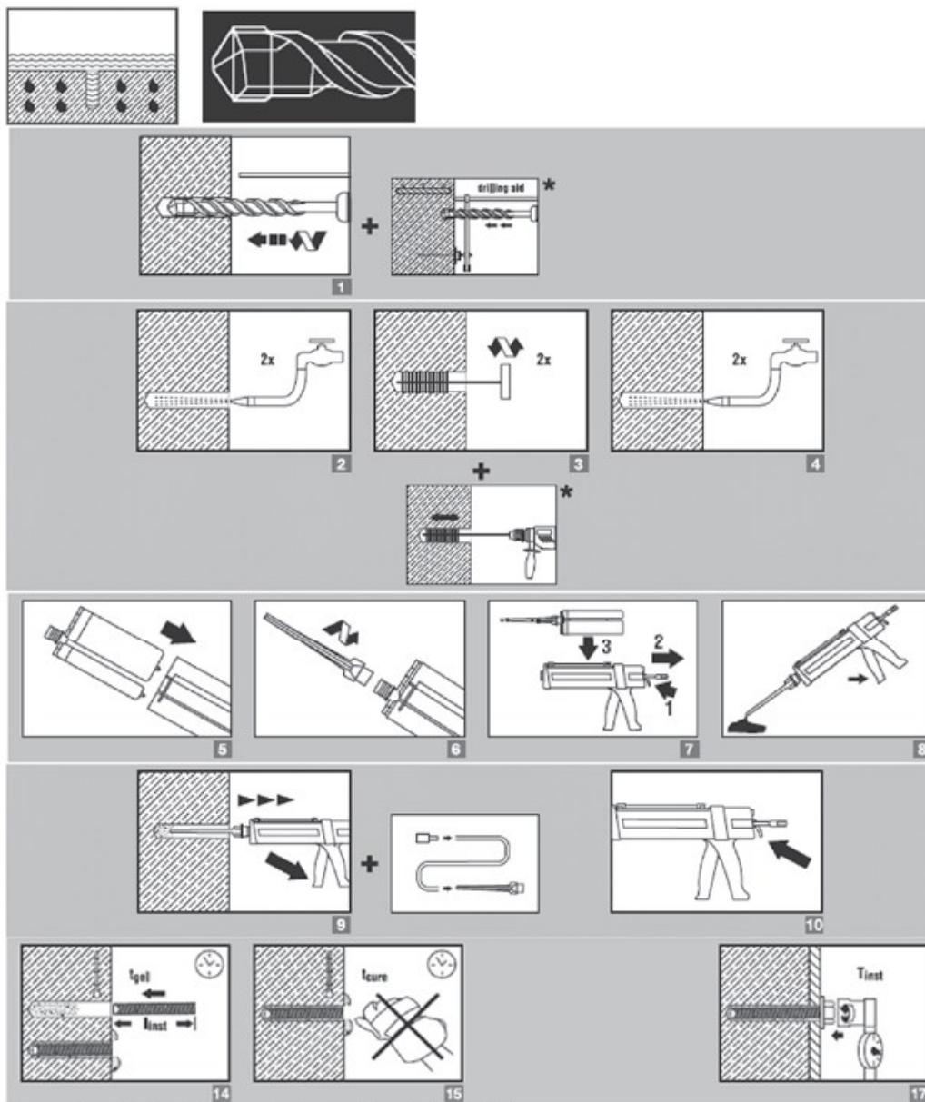
Brush bore hole with required steel brush HIT-RB
