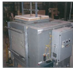
Figure 1 - Equipment used during a L-rating test.
