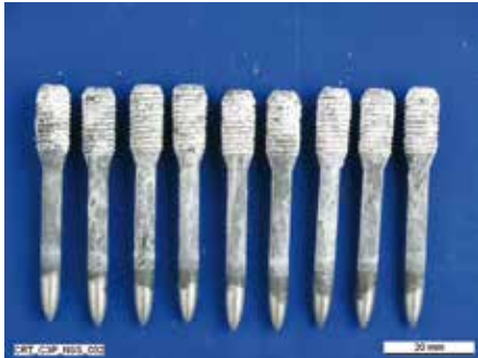
Zinc corrosion (white rust)
