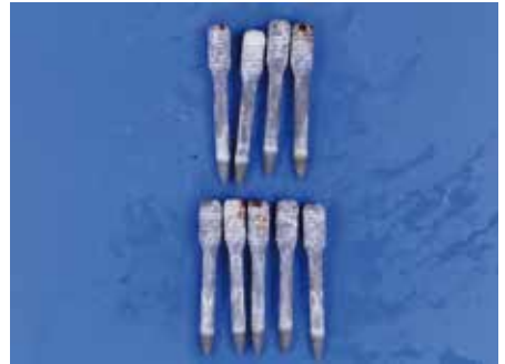
Start of carbon steel corrosion (red rust)
